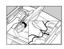
Open the Exit Guide while holding the green labeled tab.
